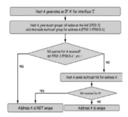
Figure.1.Duplicate Address Detection Process
