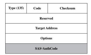
Figure.3. Modified NS Message for Safe Addressing Scheme Packet Format
